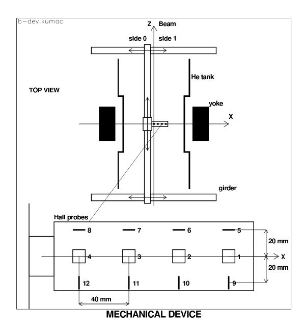
Figure 2: Mapping device
