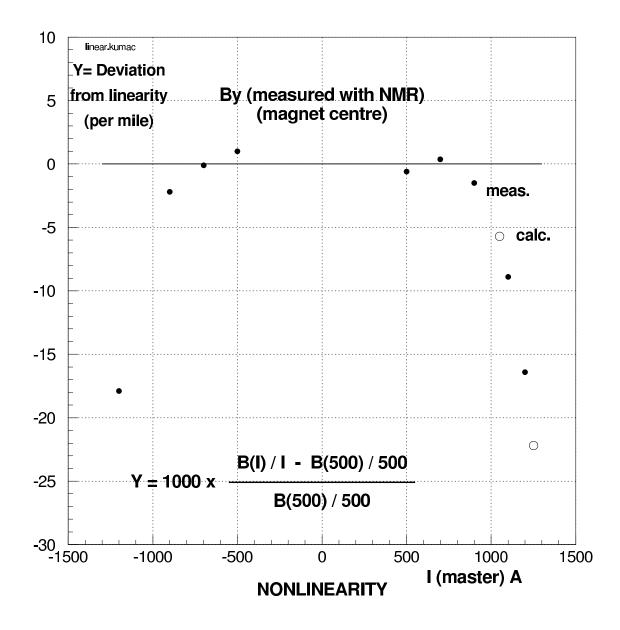
Figure 9: Saturation effect from NMR measurements
