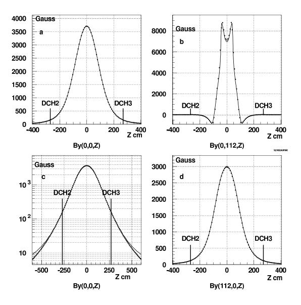
Figure 4: Plots of By vs Z, TOSCA calculations (lines) and measurement (points), without any normalization -a): x=0,y=0-b): x=0,y=112cm -c): x=0,y=0, logarithmic coord. -d): x=112cm,y=0
