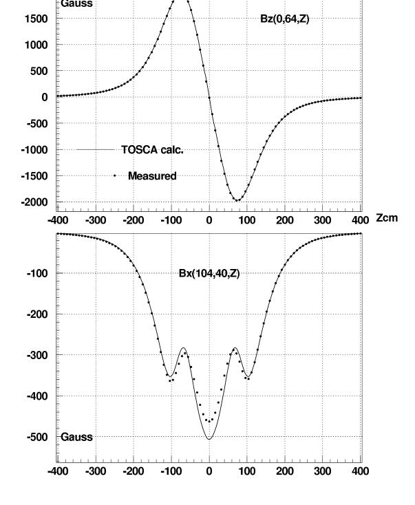
Figure 5: Plot of Bz vs z (x=0,y=64) and Bx vs z (x=104,y=40) TOSCA calculations (lines) and measurement (points)
