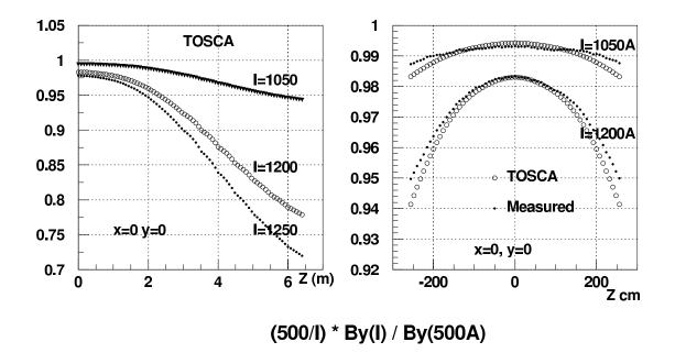
The saturation effect is small about 2% for small z Effect Larger than 20% beyond z = 3m but small effect on integr. field 'Quite similar effect in TOSCA and measurement, within 0.2% near the centre A difference (TOSCA-meas.) larger than 0.5% only beyond Z = 2m Suggests to use: B(I) = BT(I)\*BM(1200)/BT(1200) (BT: TOSCA BM: meas.)
