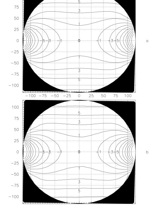
Figure 6: contours of Pt values in xy plan for calculated and measured field maps. The numbers indicate the percent deviation from the central value of Pt
