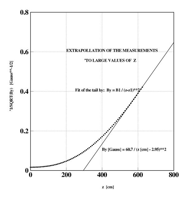
Figure 8: Extrapollation of measurements beyond -z-=6.2 m by a fit in  $1/d^**2$ . the measured magnetic field behave indeed in  $1/d^**2$  but with d=-z-3m. taking into account the final size of the magnet, source of the field.
