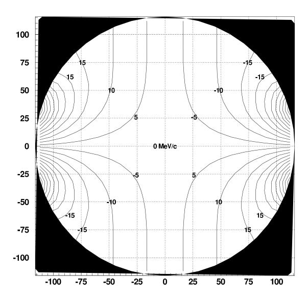
Figure 7: Contours of equal integrated field (-2.7m:2.7m) Bx, expressed as tranverse momenta (MeV/c), in the xy plan (cm), inside the He tank tube.
